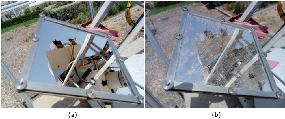
Figure 3.13: Red rain event effect: (a) TraCS mirror in a clean state; (b) TraCS mirror after red rain event.
