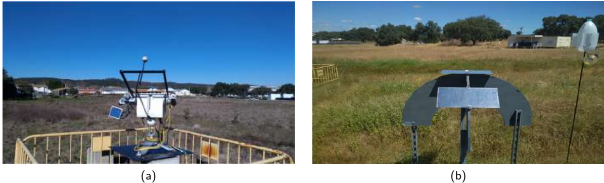
Figure 5.1: Measurements setup: (a) TraCS; (b) Modified glass tree.
