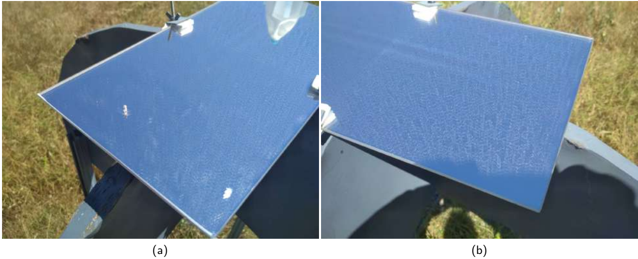
Figure 5.4: Uncoated and coated sides of the horizontal mirror a few days after the first cleaning: (a) Uncoated; (b) Coated.
