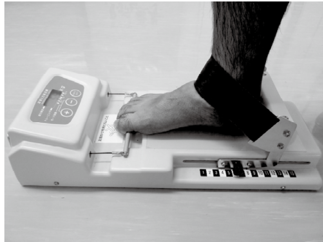
Figure 3 Measurement of toe grip strength
