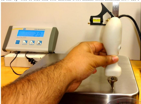
Skin Pitch reference measurement when skin plane is aligned with the Earth Horizon
