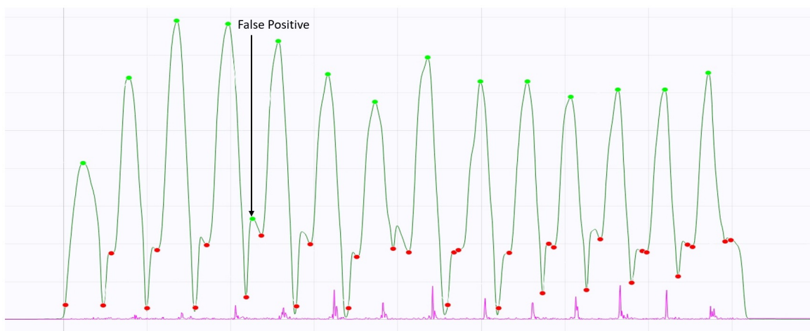
Fig. 9.9.: Treatment Strokes with corresponding peaks yielded from the redundant peak filtering algorithm
