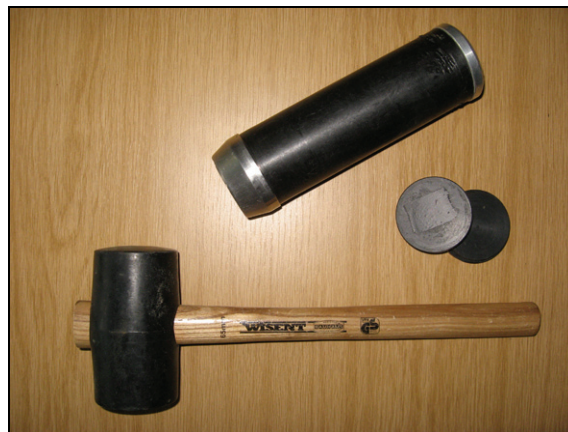
Figure 05: OSL sampling equipment consisting of an opaque plastic tube equipped with cutter (top), opaque plastic caps to seal the tube after sampling (middle) and soft hammer for driving the tube into the sediment (bottom).
