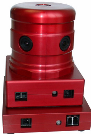
Figure 1. The Ladybug camera used for recording lectures in the classroom. The system consists of five cameras arranged radially, and sixth camera pointing up. The six cameras cover 70% of a spherical view centered at the system.
