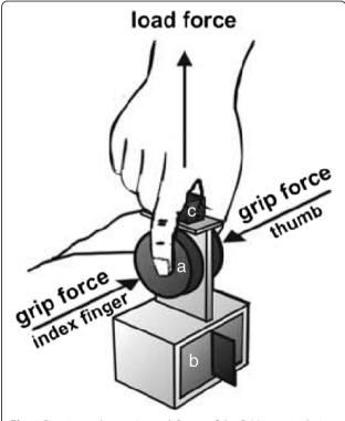
**Fig. 1** Experimental setup. Legend: Set-up of the Q-Motor grip device (**a**) force transducers for measuring the grip forces of the thumb and/ or index finger (*here thumb*), (**b**) the exchangeable weights (250 g or 500 g), and (**c**) the 3D position sensor for measuring involuntary movements
