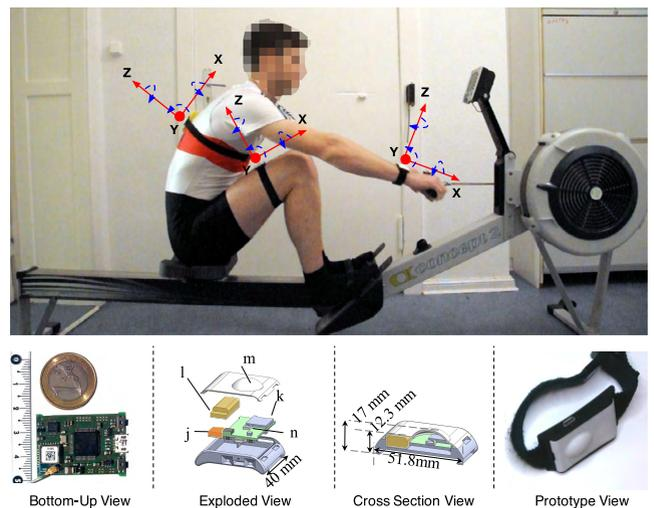
FIGURE 5. Hardware setup. (top) Placement. (bottom) Node configuration.
