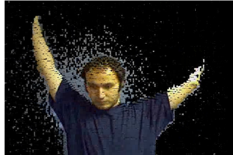
Figure 6. Noise introduces a depth-measurement error of up to 30 cm. Which makes a segmentation exclusively by depth-range checking impossible.
