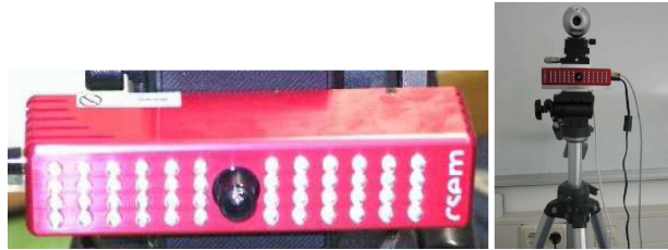
Figure 2. The Swissranger SR-2 3D-camera (left picture) and the 2D/3D-camera combination mounted on the self-developed pod (right picture).
