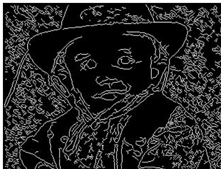
Figure 10. Resulting image of the canny algorithm.
