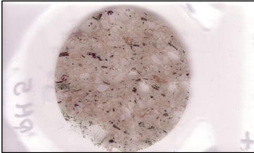
PM-6 (553069/7486426): Similar to PM-5. Fine grained crystalline matrix with fluidal texture. Medium sized (~4 mm), subangular phenocrysts of plagioclase, alkali feldspar, hornblende, biotite and quartz. Elongated pumice fragments. No shock features; strong alteration, also indicated by the alteration of glass to chlorite.
