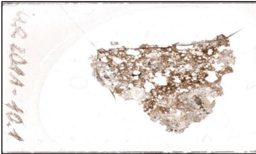
UR-2011_10a (551829/7483040): Different melt phases including translucent glass, brownish schlieren, and small black glass particles. Vesicle rich. Quartz (with PDF) and feldspar occur in lithic clasts.
