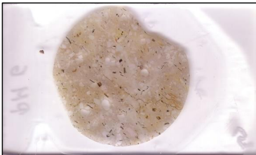
PM-6 (553069/7486426): Similar to PM-5. Fine grained crystalline matrix with fluidal texture. Medium sized (~4 mm), subangular phenocrysts of plagioclase, alkali feldspar, hornblende, biotite and quartz. Elongated pumice fragments. No shock features; strong alteration, also indicated by the alteration of glass to chlorite.
