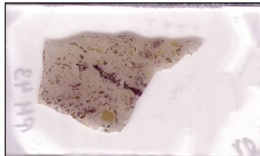
PM-46 (541662/7478993): Fine grained crystalline matrix with fluidal texture. Medium sized (~4 mm), subangular phenocrysts of alkali feldspar, hornblende, plagioclase, biotite, and quartz. Some pyrite grains. Elongated, vesicle-rich pumice fragments with interfingering contacts. Strong alteration with sericitisation of feldspar and chloritisation of biotite and hornblende.
