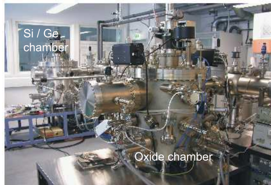
FIG. 6: UHV System containing three MBE deposition and one analysis chamber, interconnected with a linear transfer system
