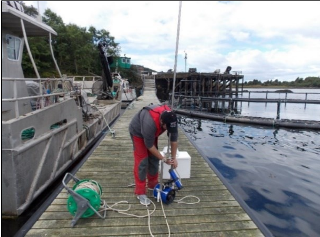
Figure 3.6 Fish around cages were recorded using a standstill underwater camera system mounted in a housing operated by attaching poles and a rope to the desired depth
