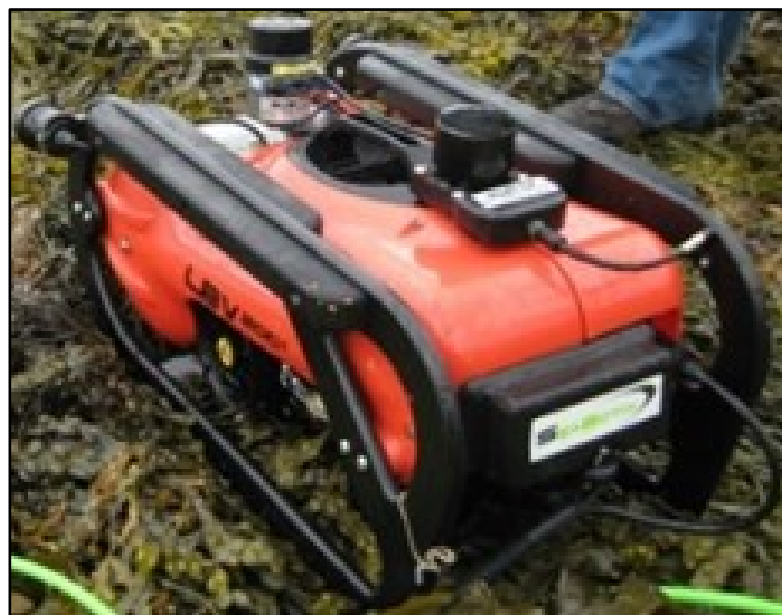
Figure 3.5 Several trials were conducted to record fish around cages using a remotely operated vehicle (ROV).
