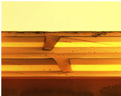
Fig. 13. Cross section of an interplane turning-mirror configuration in Ormocer material where the light signal undergoes a double 90^\circ bend with change of the propagation direction.
