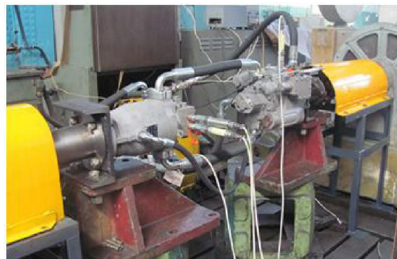
Fig. 4 – Appearance of stand №2 for studying HST
