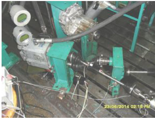
Fig. 2 – Appearance of stand №1 for studying HST
