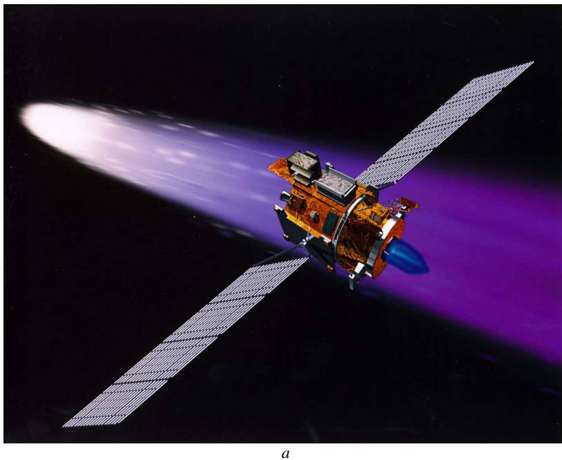
Fig. 3 – Spacecraft Deep Space 1 (NASA, 1998) ion engines using xenon: a – Deep Space 1 spacecraft against the background of Borelli’s comet; b – preparation for installation in the launch vehicle DELTA II, McDonnell Douglas, USA.
