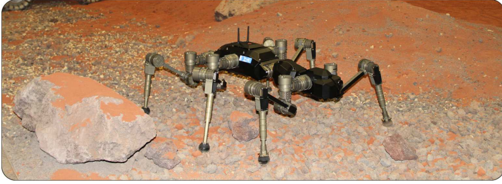
Figure 2.13: The SPACECLIMBER system in an environment simulation the Mars surface.
