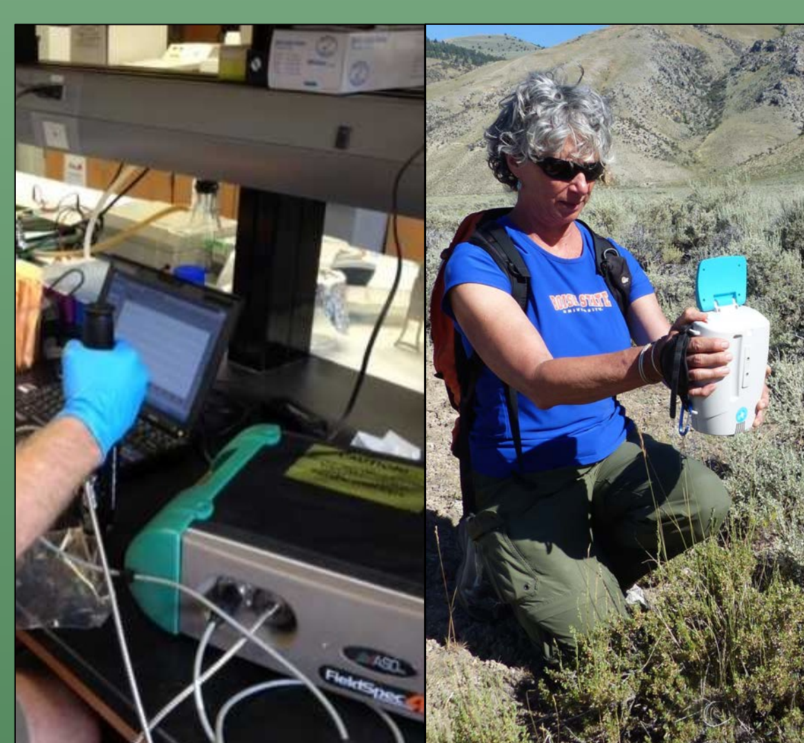
Fig 1. Examples of handheld spectrometers measuring near infrared spectroscopy (NIRS)
