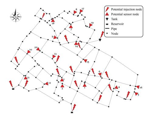
Fig. 1. Lamerd City's Water Distribution System. Potential locations for placement150
