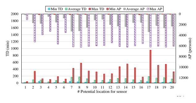
Fig. 3. Minimum, average and maximum time to detection (TD) at potential335locations for sensor placement; and minimum, average and maximum affected336
