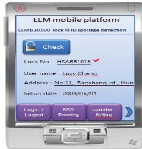
Figure 8. Front-end Mobile Device Interface of the Lock System - RFID Spoilage Detection Module
