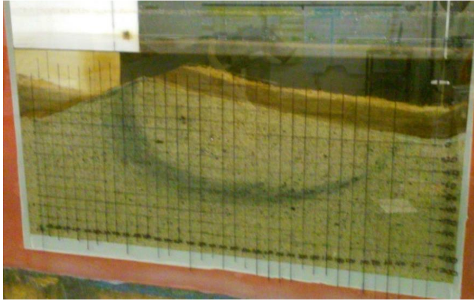
Figure 4.3. Cross-sectional view of a 70 cm dune in F2. The grayish streak developed over the duration (91 days) of the experiment. Surface water flow is from right to left. The black grid lines are spaced at 1 cm.
