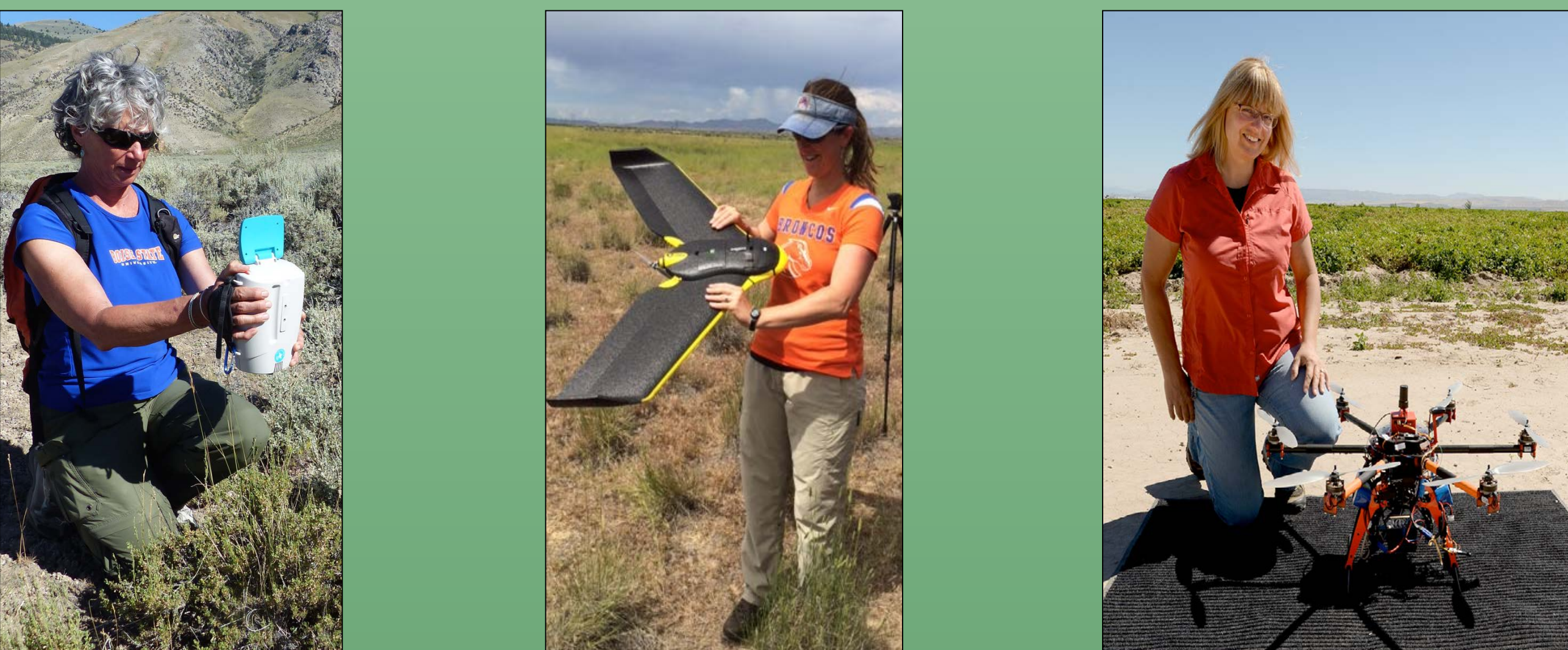
Fig 1. Examples of spectrometers on handheld devices (left) and attached to unmanned aerial systems (middle, right).
