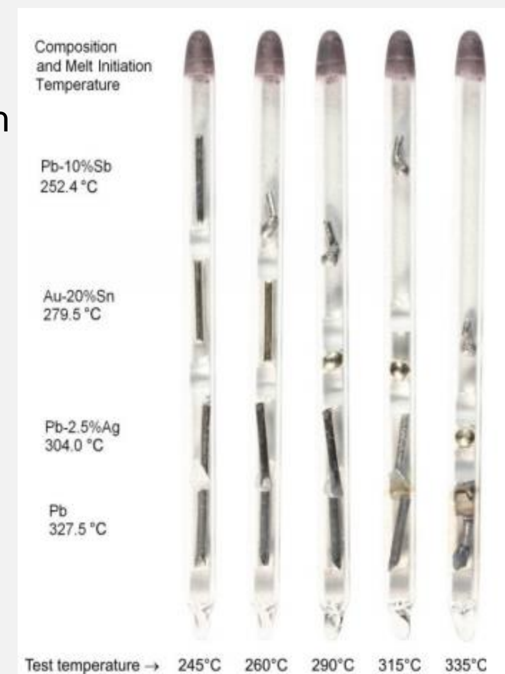
Fig. 1. Melt wire techniques [1].
