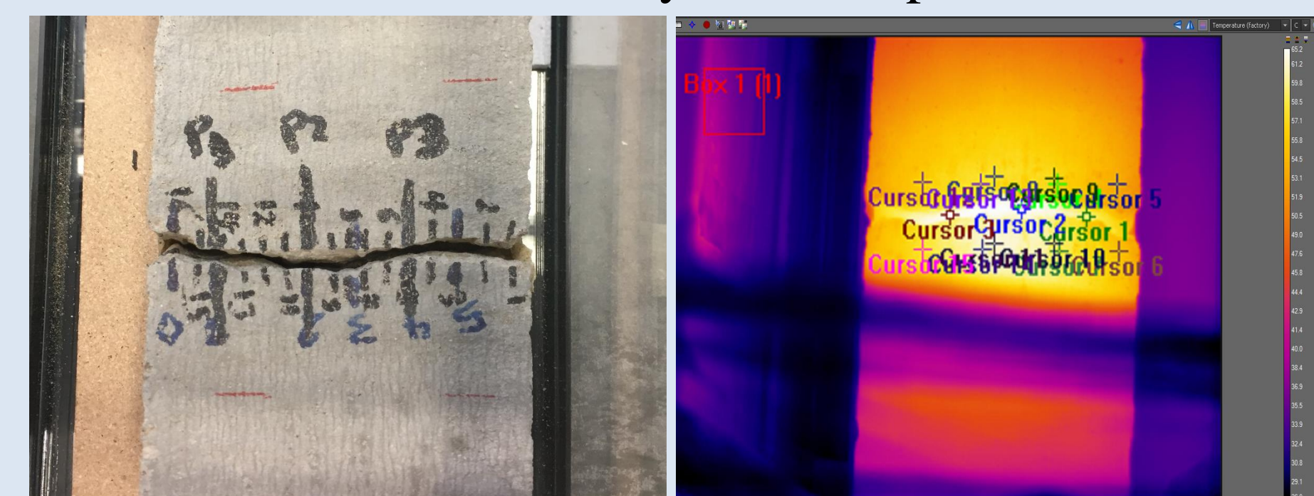
Thermal image of concrete in ResearchIR
