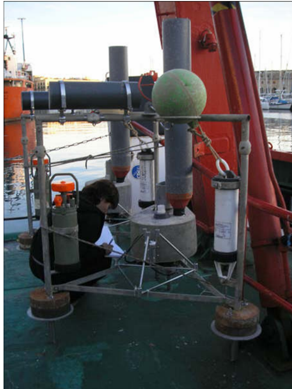
Figure 2.2. Picture of the benthic tripod used in this project.
