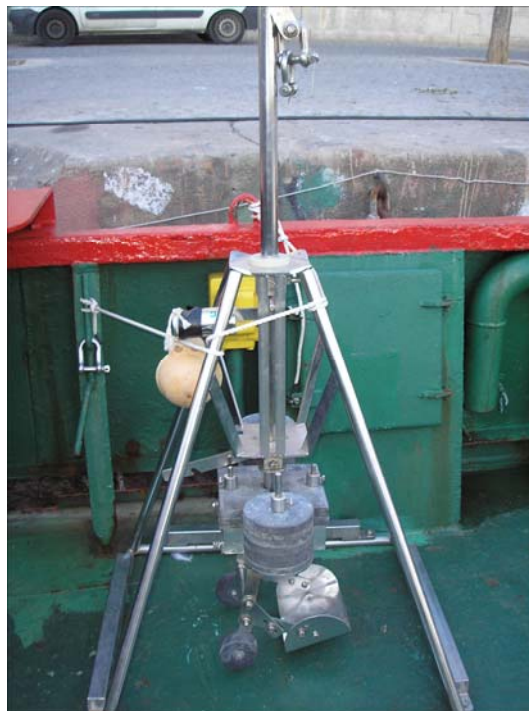
Figure 2.6. Picture of the box corer used in this project (model Haps corer by KC-Denmark).
