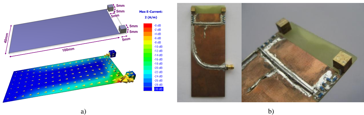
Fig. 1.18 a) Geometry and dimensions associated to the radiating structure, as a first solution of this thesis development comprising two non-resonant ground plane boosters, each one in charge of the ground plane excitation for each frequency region. Current distribution referred to the excited ground plane mode at f=0.892\text{GHz} ; b) Prototype associated to the geometry shown in a).
