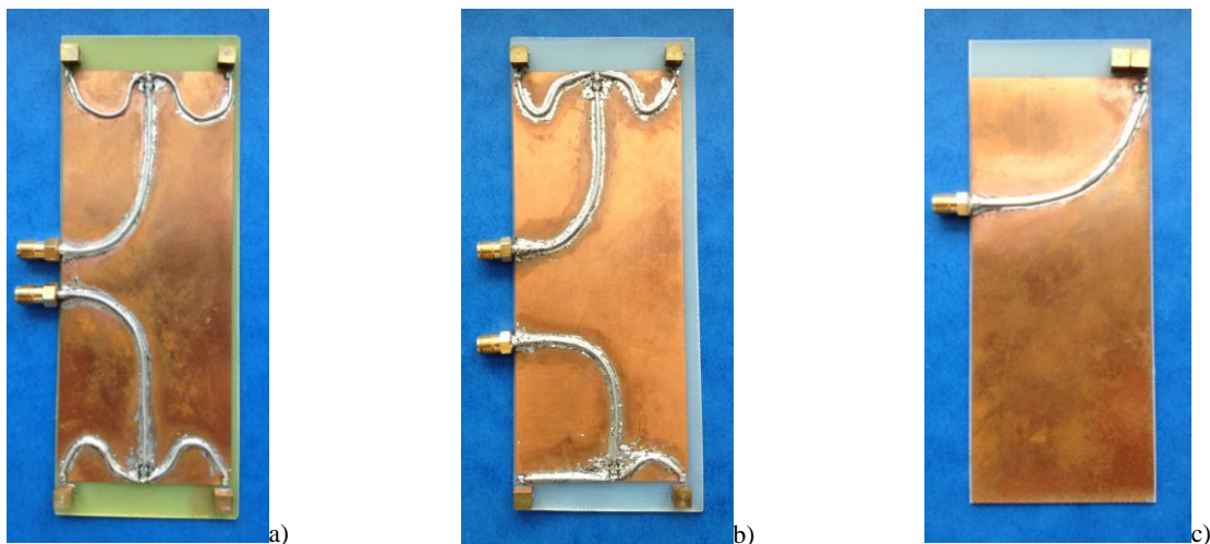
Fig. 5.44 Prototyped solution including a) in-phase feeding scheme for both frequency regions; b) in-phase feeding scheme for the LFR (upper edge) and out-of-phase feeding scheme for the HFR (bottom edge); c) Single element 5 mm x 10 mm x 5 mm with a broadband matching network (note that for the single element case the component values of the matching network are adapted according to the frequency region of operation). The reactive elements used are SMD0402.
