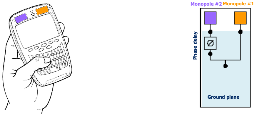
Fig. 5.1 Schematic example of a distributed antenna system consisting of a passive array of two monopole antennas placed at the corners of the ground plane of a handset device. A phase delay \phi is used to optimize the bandwidth.
