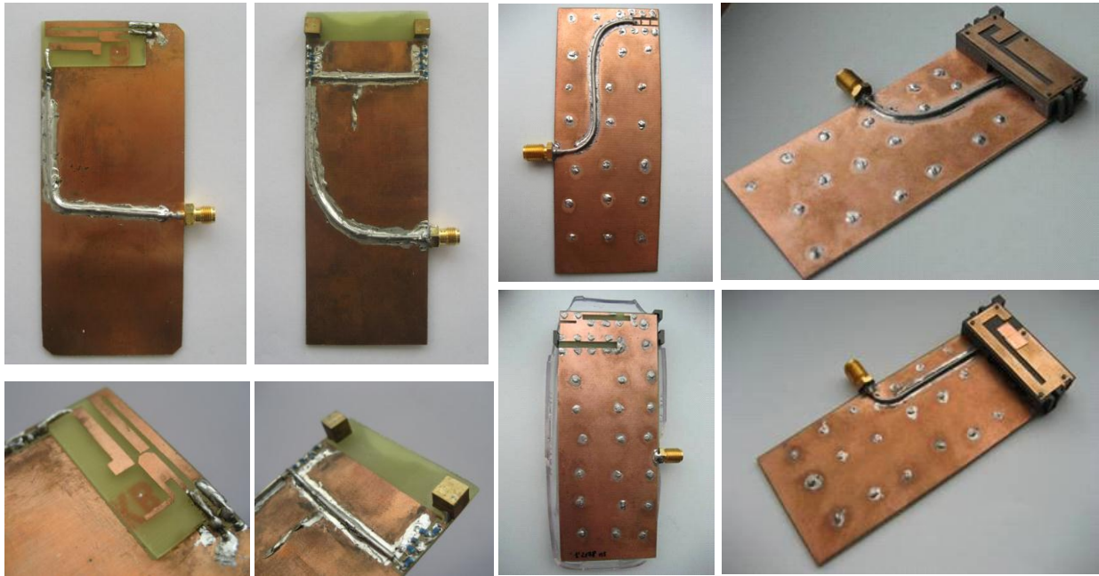
Fig. 4.1 Geometry of the four radiating systems proposed. All prototypes are etched over a 1 mm thick FR4 piece ( \epsilon_r=4.15 , \tan\delta=0.013 ). Penta-band coupled monopoles set (left), penta-band compact radiating system (2 nd column), dual-band PIFA (top right), and hexa-band PIFA with a slotted ground plane (bottom right).
