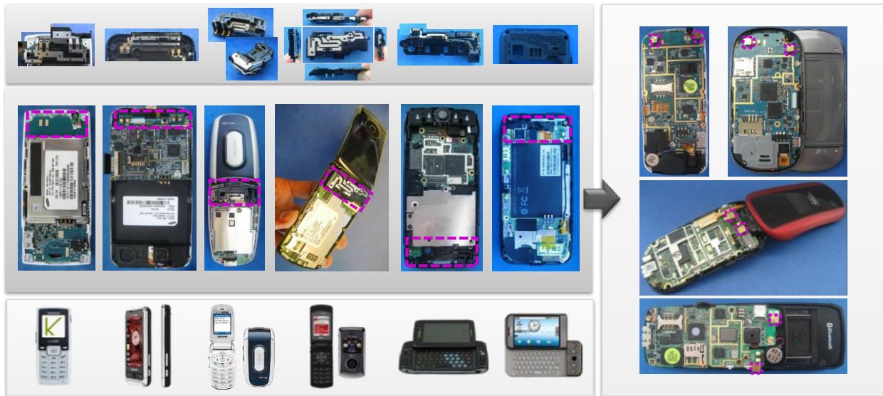
Fig. 1.10 Left: Example of several handset platforms featuring different form factors and consequently dissimilar internal antennas especially customized for being integrated in such specific handset platforms; Right: Ground plane booster elements as the promising standard solution that enables the integration in any handset platform without the need of a complex customization process.
