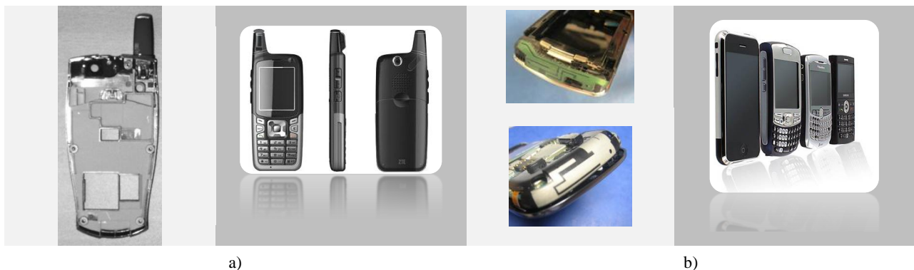
Fig. 1.1 Handset antenna evolution: a) Example of an external antenna and a handset including such external antenna; b) Example of two internal antennas and handsets including internal antennas.
