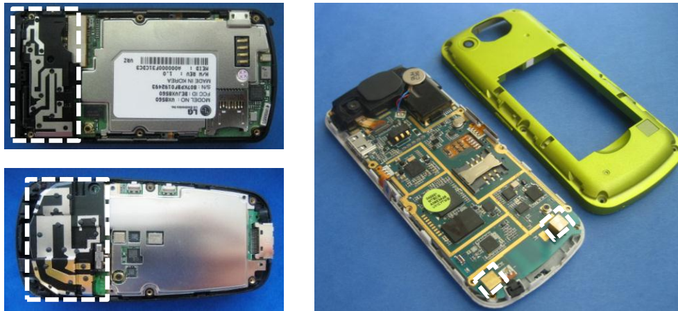
Fig. 1.9 Comparison between current internal antenna technologies and the technology proposed in this thesis. Note that the PCB space is considerable increased when the dedicated antenna (framed in dashed line (left)) is replaced by the non-resonant ground plane boosters (framed in dashed line (right)).
