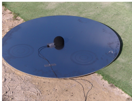
FIGURE 5.3: True flush surface microphones used for the experimental validation of the acoustic method for aircraft localization.
