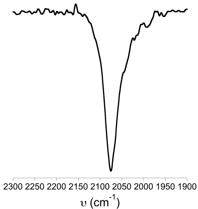
Figure 4.7. IR spectra of CoHCF grown on a FTO electrode.
