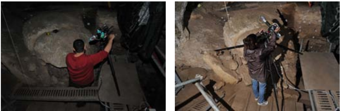
Fig. 4A.9 Using multiple viewing angles during scanning (left and right) (photos by Luis Teira).
