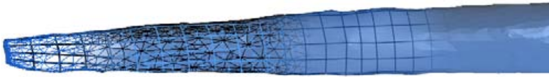
Fig. 4C.40 Detail of the FE model of wooden artefact D12_JF-JG-81. From left to right: solid mesh and elements; solid mesh, elements, and surface of the solid model; elements and surface of the solid model; surface of the solid model. It is not a solid model with a mesh on it, the mesh of elements is now the model.
