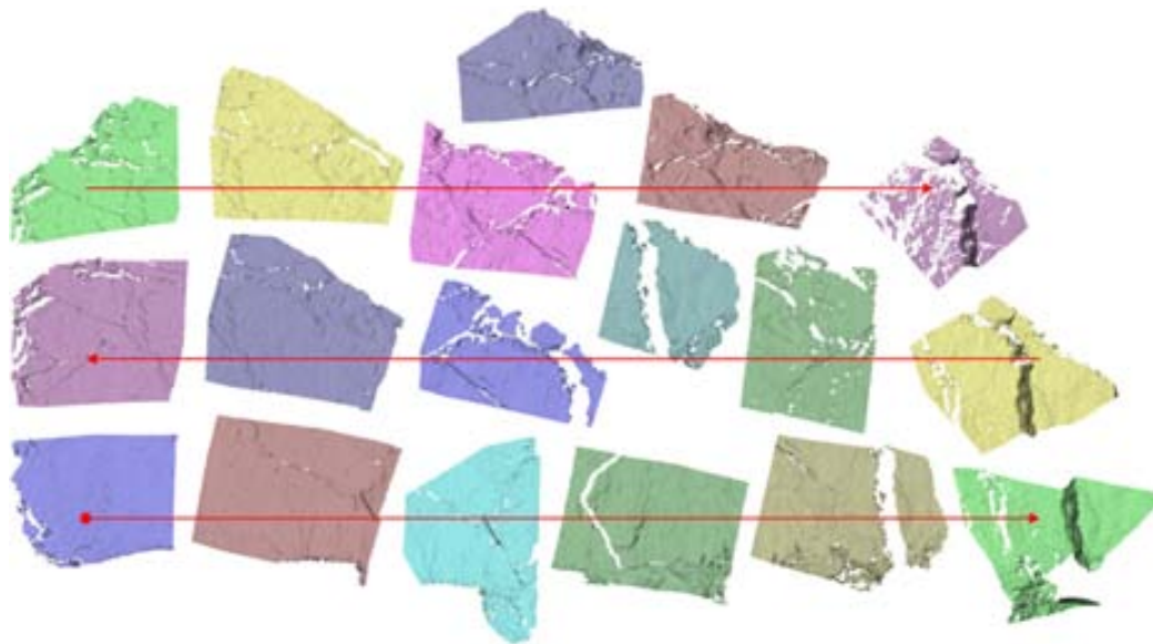
Fig. 4A.7 3D Data acquisition flow: alternation between left-right and right-left rows, and from bottom to top.
