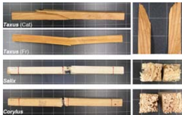
Fig. 4C.37 Static bending failures: appearance of the manner in which the failure develops (left), and the fractured surface (right) of the tested specimens (photos by Antonio Nadal).
