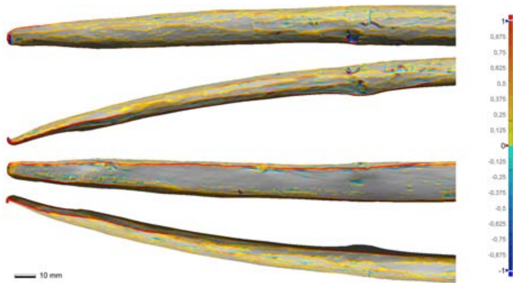
Fig. 4C.25 Curvature analyser colourmap of artefact D12_JF-JG-81: detail of end D. Back, left side, belly, and right side views (from top to bottom). 150 mm FOV: maximum curvature -0,2/0,2 with allowable value hidden.
