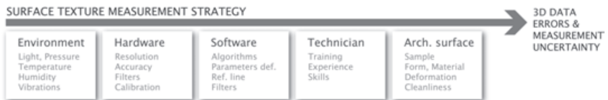
Fig. 3.9 Example of sources of measurement error in surface texture that lead to uncertainty of measurement results.
