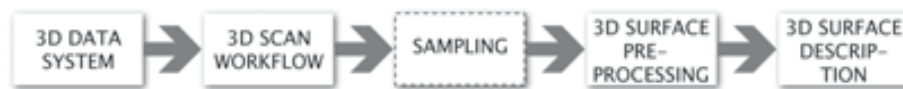
Fig. 3.8 3D Surface texture workflow: from choosing a 3D data acquisition system to describing the 3D digital surface texture.
