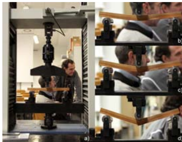
Fig. 4C.35 Static bending (flexural) test: course of the deformation and fracture of specimen Tfr-33, Taxus baccata .
