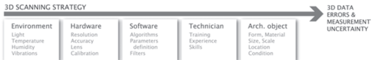
Fig. 3.5 Example of sources of measurement error that lead to uncertainty of measurement results.
