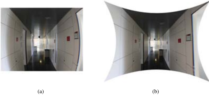
Figure 2.3: Original image and image with distortion compensated. As can be seen in (b), in the periphery zones of the compensated image the walls remains straight.
