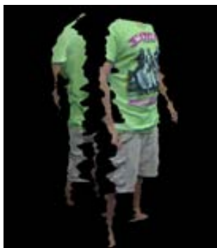
Figure 5.6: Frontal mesh and back-right mesh. Views are intentionally separated in Z axis for better comprehension.
