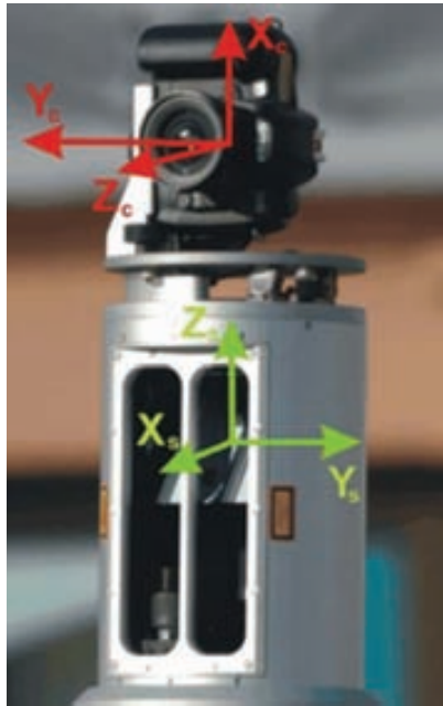
Figure 2.4: Coordinate system for the 3D scanner and for the visible camera.
