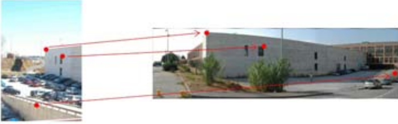
Figure 3.1: Point correspondences between two images representing a similar scene from different viewpoints. In addition to these visual images, it is expected that the corresponding range images were also available. The combination of these point correspondences determine a rigid transformation between the 3D structures.
