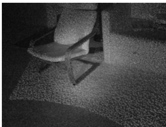
Figure 1.6: Infrared pattern projected by the Microsoft Kinect device.
