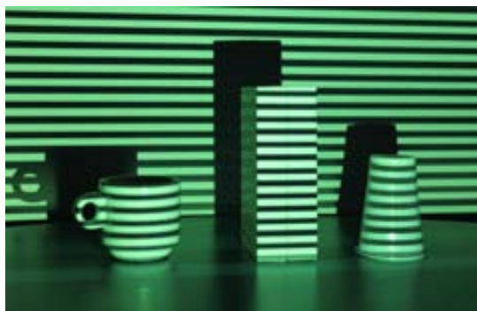
Figure 1.5: Pattern of structured light composed by a static set of lines. The shape produced by the illumination in the objects make possible the estimation of their 3D point cloud.
