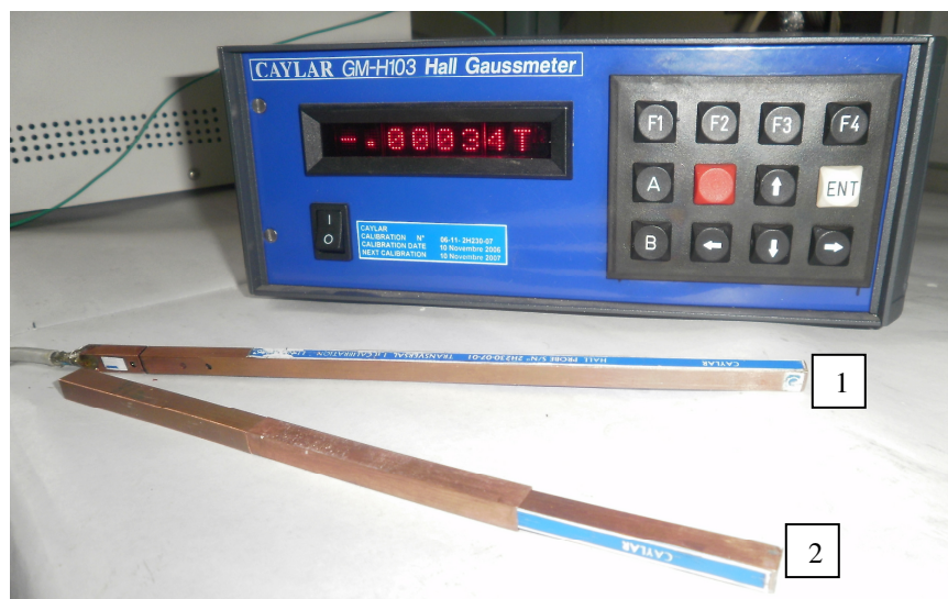
Figure 45: Caylar GM-H103 Gaussmeter with transverse (1) and axial (2) Hall probes.
