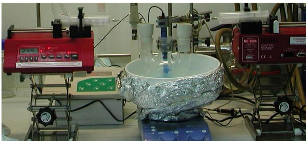
**Figure II. 9.** Reaction set-up for the epoxidation of **112a**.
