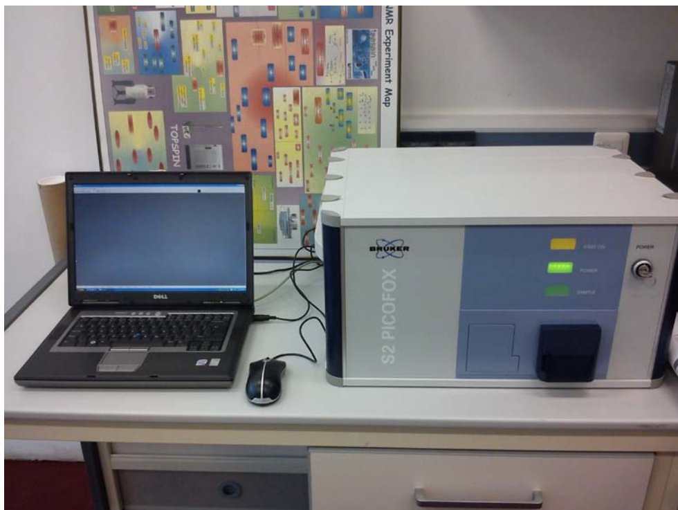
Figure 1.7. A benchtop total reflection X-ray fluorescence (TXRF) spectrometer “S2 PICOFOX”.
