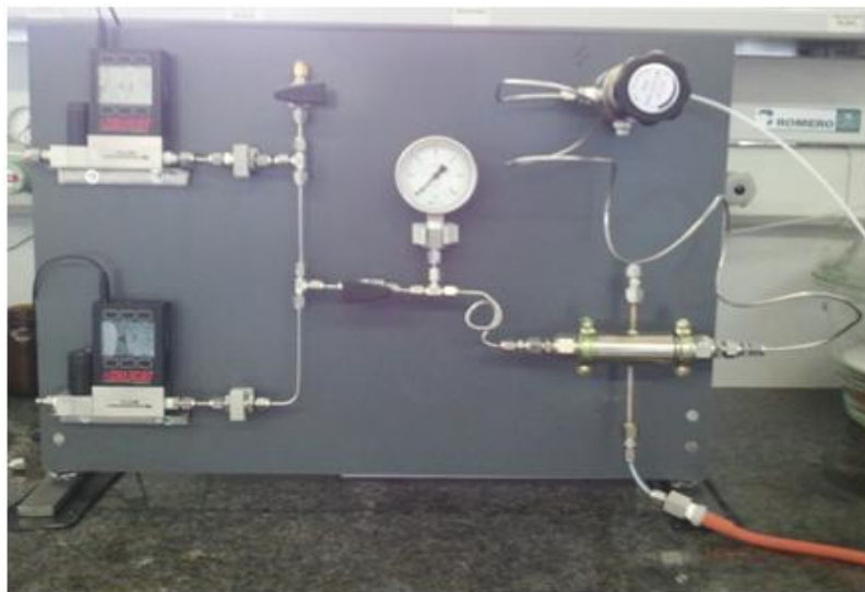
Figure III. Set-up for testing the membrane permeance employed in METEOR research group, URV, Tarragona, Spain.
