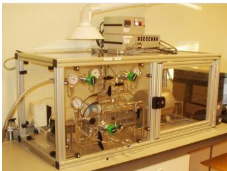
Figure V. Set-up for testing the membrane permeance employed in IM group, University of Twente, Holland.
