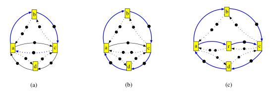
Figure 4. (a) A back-pressure graph; (b) The capacity of (a, c) is resized to 3; (c) One buffer is inserted in (a, c).
