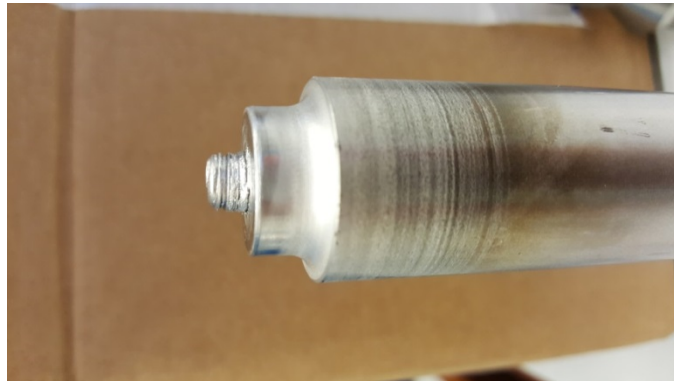
Figure 7. Circular threaded pin. Geometry detail.
