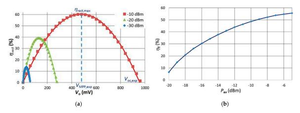
**Figure 4.** (a)  $\eta_{\text{rect}}$  versus  $V_0$  for different values of  $P_{av}$ . Continuous lines are least-squares fits corresponding to a Thévenin equivalent circuit; (b)  $\eta_{\text{T}}$  versus  $P_{av}$ .
