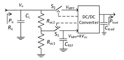
Figure 3. Block diagram of an implementation of the FOCV-MPPT technique.
