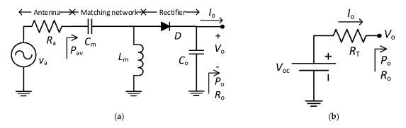
Figure 2. Rectenna: (a) Schematic circuit; (b) Thévenin equivalent circuit.
