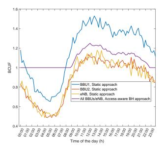
Figure 3: System BCUF during 24 hours with 80% system backhaul capacity.
