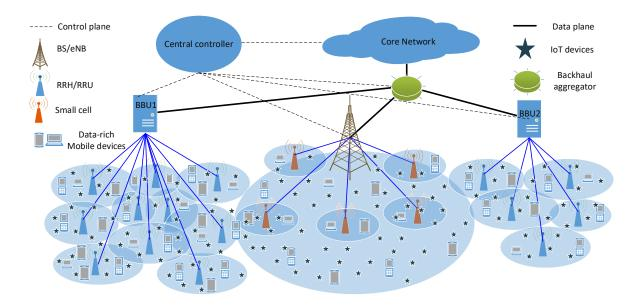
Figure 2: Heterogeneous 5G scenario with 2 BBUs and 1 eNB covering  $1km^2$  area.
