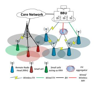
Figure 1: Complex heterogeneous backhaul in 5G networks..
