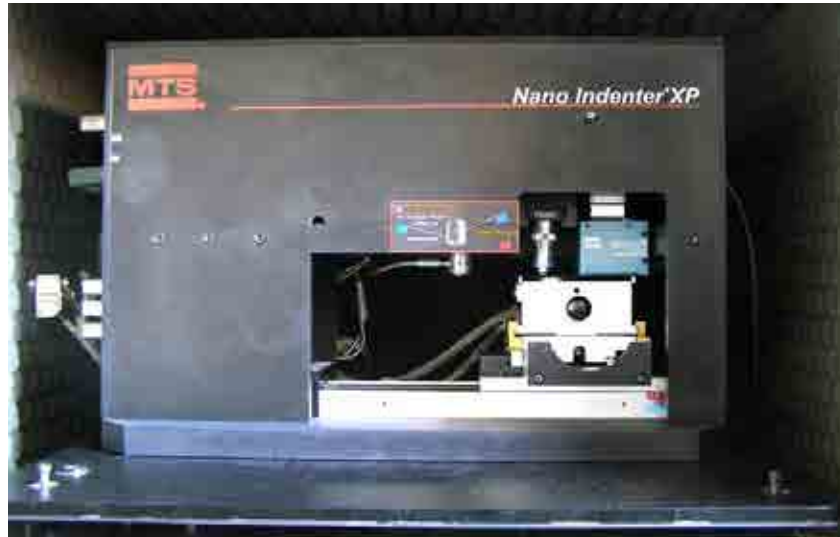
Figure 12. Nanoindentation equipment used for the mechanical characterization.
