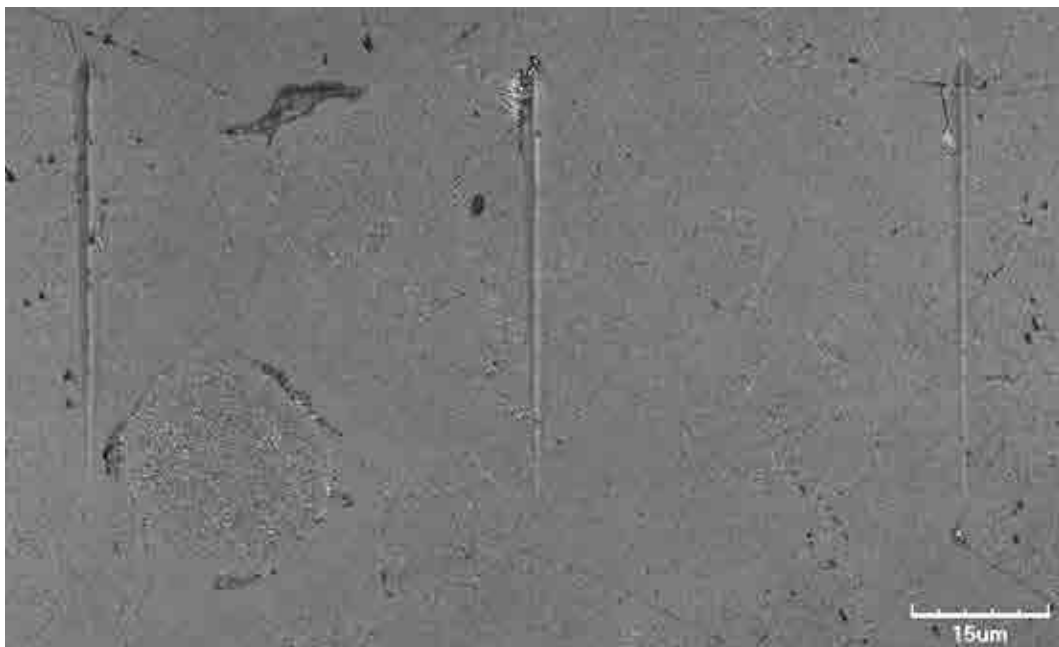
Figure 9. Three low load scratches performed on sample M5 . Scratches are positioned vertically in the micrograph, with the applied load increasing upwards.
