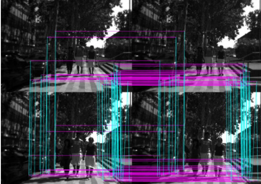
Figure 2.1: SIFT correspondences in two consecutive stereo image pairs after outlier removal using RANSAC.
