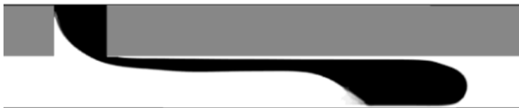
Figure 8.5: Thread generation without squeezing. U_{SL} = 0.318 \text{ m/s} and U_{SG} = 0.182 \text{ m/s} .
