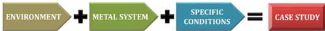
Figure 2.10: Important points to take into account when a corrosion resistant material is to be designed.
