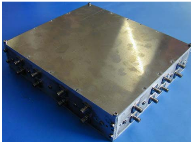
Figure 7.9: 2.7 GHz power combiner housing box. Two combiners are stacked in this box, one for each polarization, hence the paired SMA connectors
