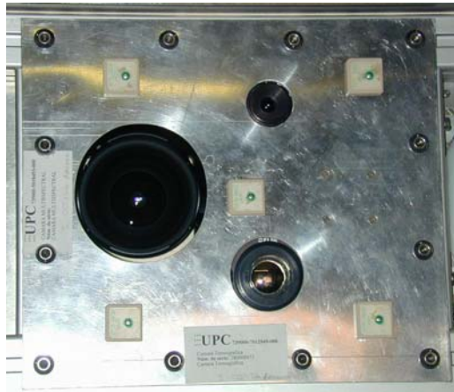
Figure 7.19: Front view of the three cameras present in the MERITXELL radiometer. The camera at the top is the IP camera, the camera at the left is the multispectral camera, and the camera on the bottom is the IR camera.
