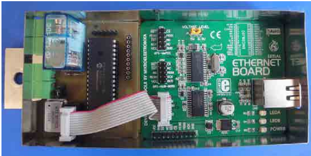
Figure 7.20: Microchip 16F877A PIC and Ethernet controller board.
