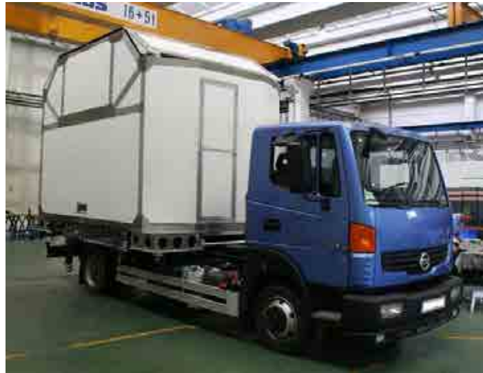
Figure 7.4: Mobile unit's housing mounted over the truck
