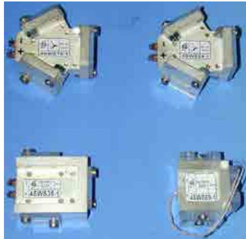
Figure 7.10: Latching circulators for the 18.7 to 89 GHz frequency bands.
