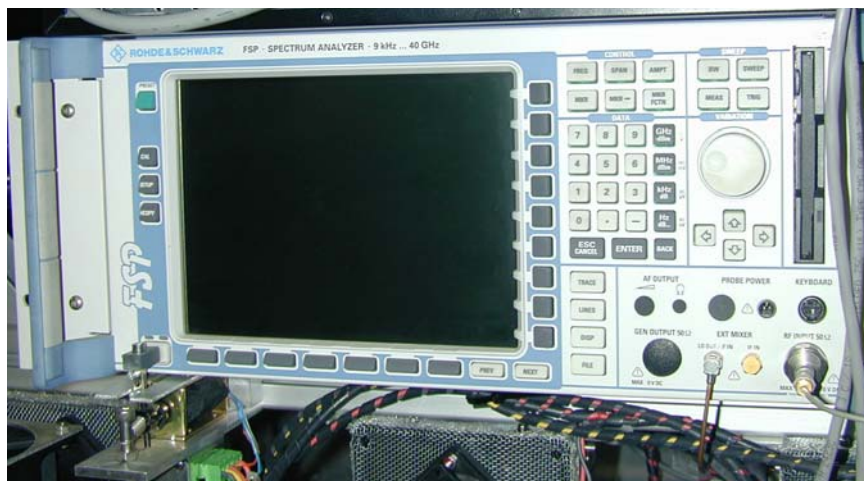
Figure 7.18: Front view of the FSP40 Spectrum Analyzer, note the two RF inputs, left one corresponding to the down-converted W-band and right one corresponding from DC to 40 GHz.
