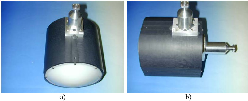
Figure 7.6: 36 GHz lens antenna. a) front view; b) lateral view
