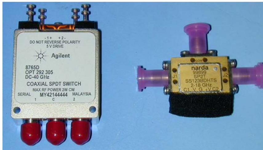
Figure 7.15: Switches used for the polarization switching: (left) D.C. to 40 GHz switch and (right) 2 GHz to 18 GHz switch for the IF signal coming from the W-band.
