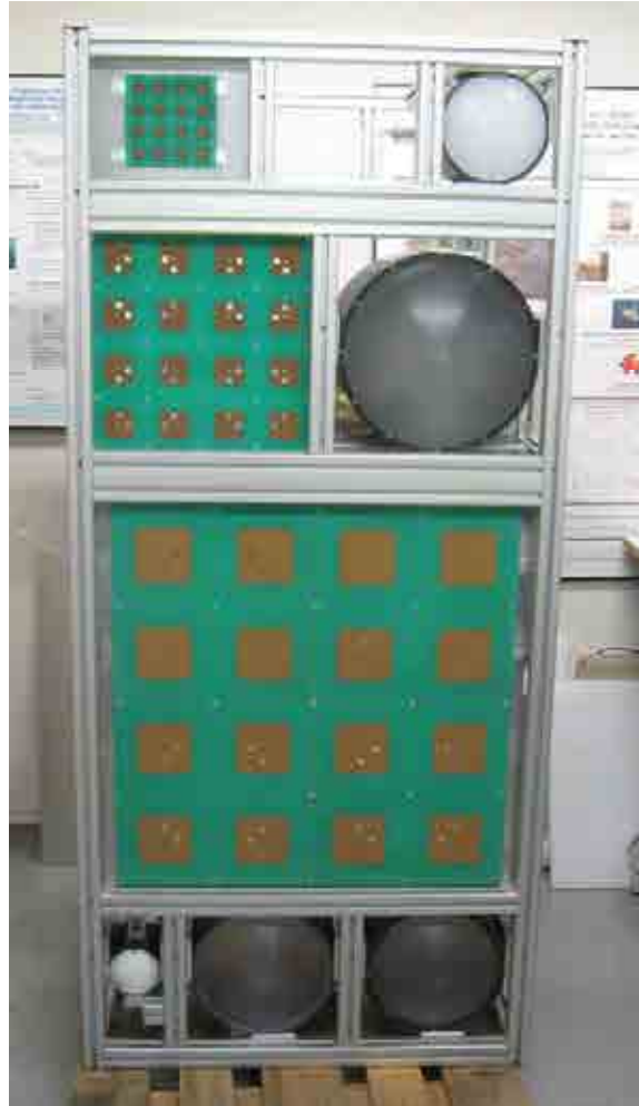
Figure 7.30: Aluminium internal structure of the MERITXELL radiometer with the horn and the patch antennas.
