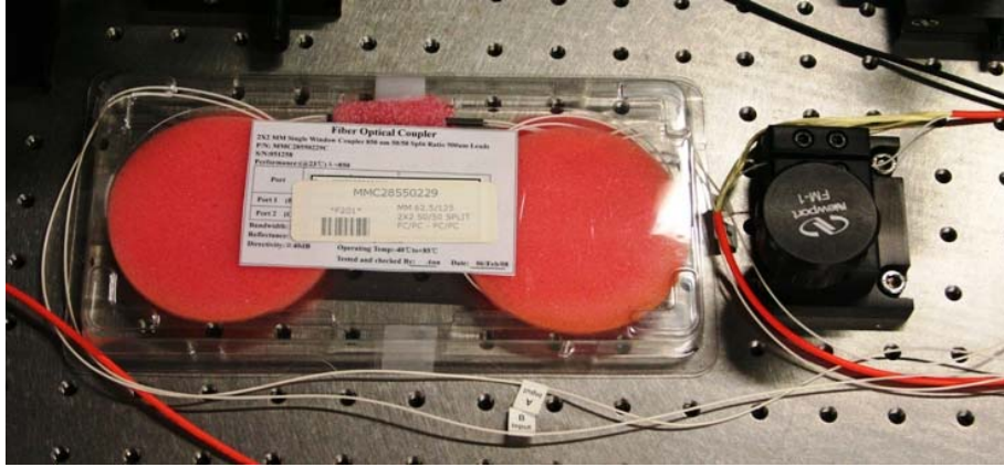
Fig. 50. 2x1 coupler and mode scrambler.
