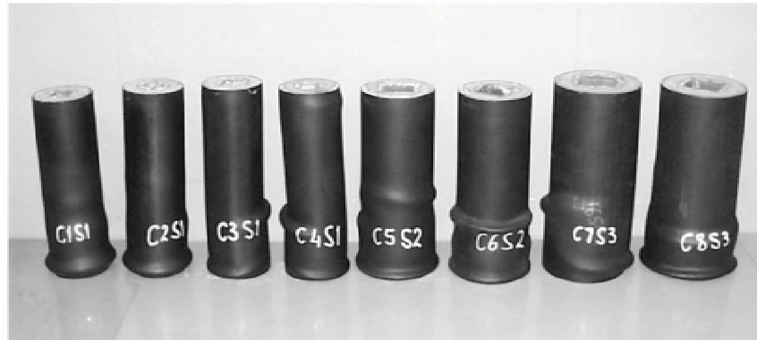
Fig. II.37 Collection of tested CFDST specimens with circular and square inner tubes. (Elchalakani, et al., 2002)
