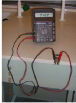
Figure 18. Schematic representation of surface resistance measurement between two electrodes
