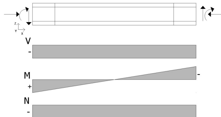
Figure 3.27 – Internal forces in the beam specimens VN2 ( N=0 ) and VN4 ( N=1\text{MN} ) by Kaufmann and Marti
