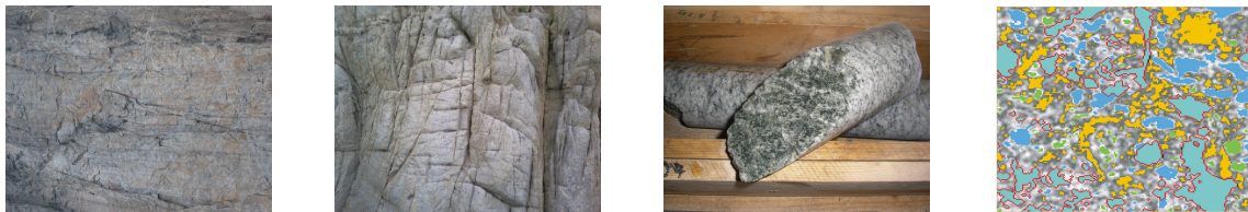
Figure 1.1: Example of heterogeneity at different scale. From the left: fracture granite formation at km scale, fracture granite formation at m scale, sample of granite at cm scale, X-ray microtomography of Majorca limestone (Courtesy of Philippe Gouze, CNRS Montpellier).
