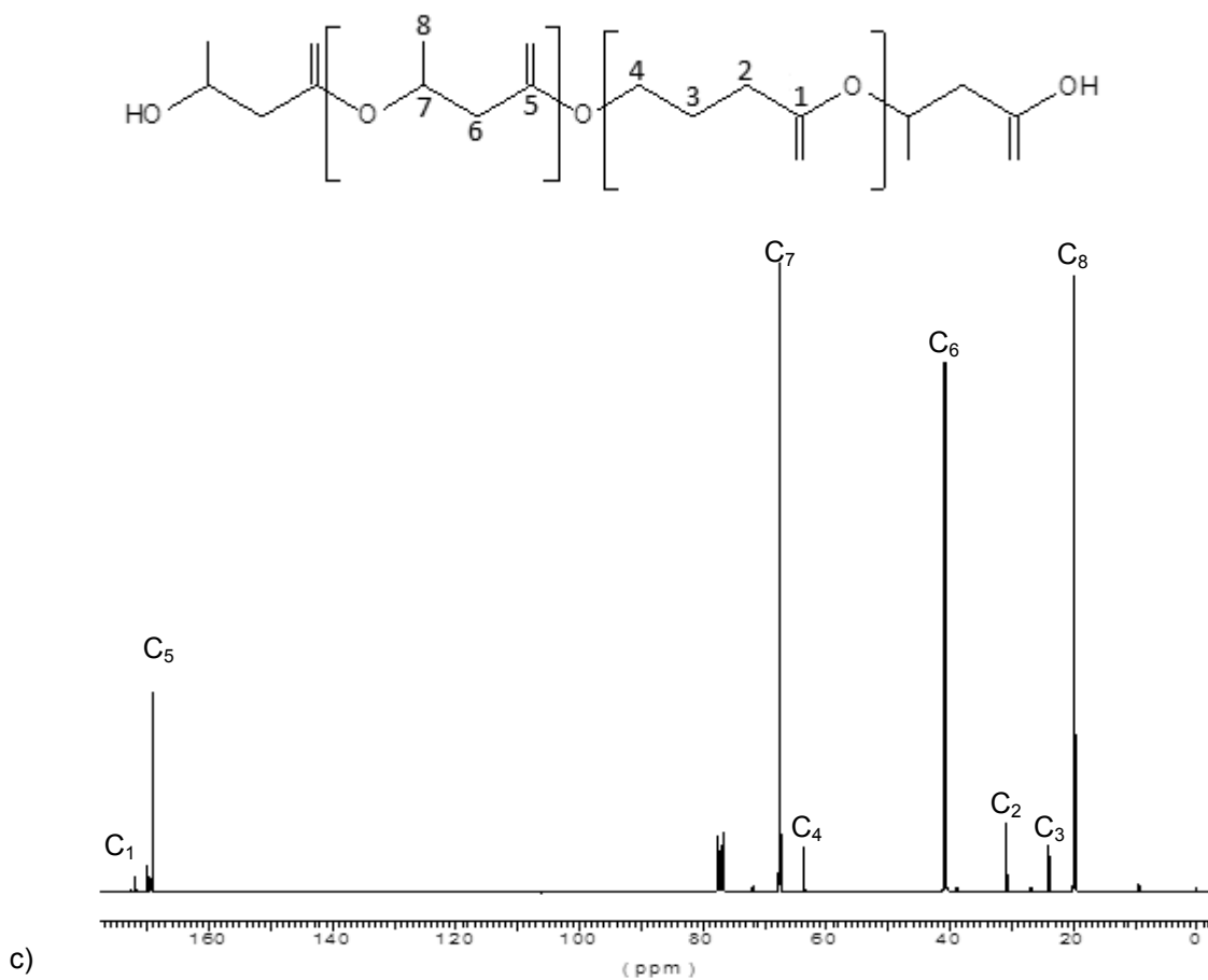
Figure 4. P(3HB-co-4HB) chemical structure. ^1\text{H} NMR spectra of P(3HB-co-4HB) samples degraded with LA (a) and LB (b). ^{13}\text{C} NMR spectra of initial P(3HB-co-4HB) (c)
