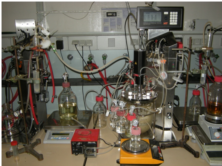
Figure 10. Photography of a 3L-Bioreactor while producing PHB by a novel strain
