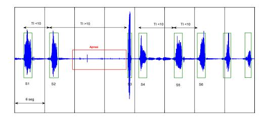
Figure 11 Excerpt of snoring sound signal. TI is the time interval between successive snores. Green boxes indicate snores episodes and the red box indicates an apnea episode.
