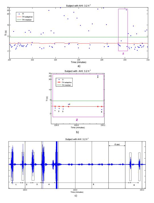
Figure 12 Performance a) (and zoom b)) of TH<sub>adaptive</sub> and TH<sub>median</sub> on an excerpt of snoring sound signal shown in c).
