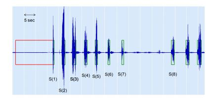
Figure 20 Excerpt of a snoring sound signal. The dashed line box corresponds to an apnea episode and the solid line boxes correspond to snore episodes. S(1) is a post-apneic non-regular snore. All S(2) - S(7) snores are regular snores. S(8) is a *normal* non-regular snore.
