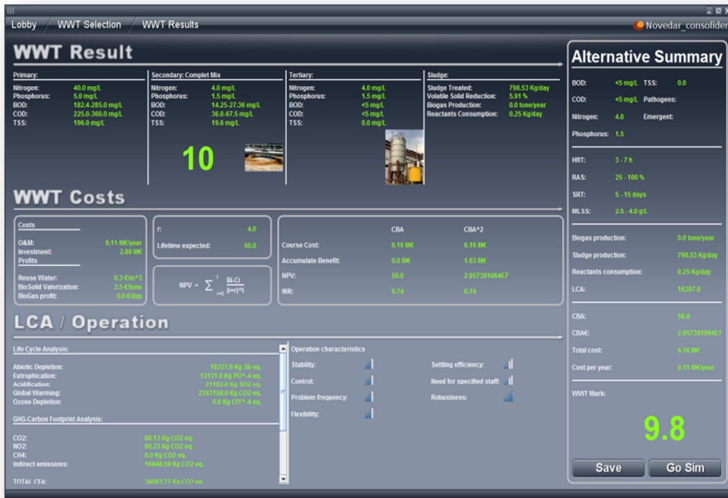
Figure 4.16. Snapshots of the results interface showing the PFD outputs for a specific scenario once the WWTP line have been selected.
