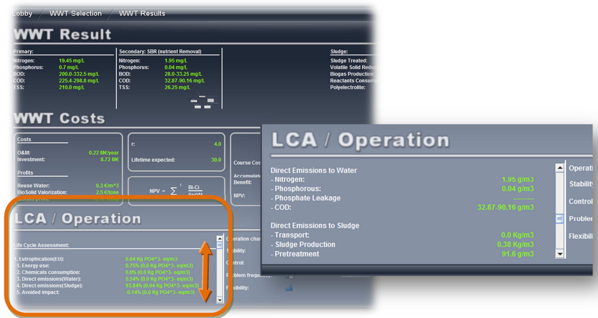
Figure 4.18. Screen capture of the EDSS. After the PFD selection a section in the summary about the LCA and its inventory is shown. A slide enables to check all these information with no need to close the results or summary window.
